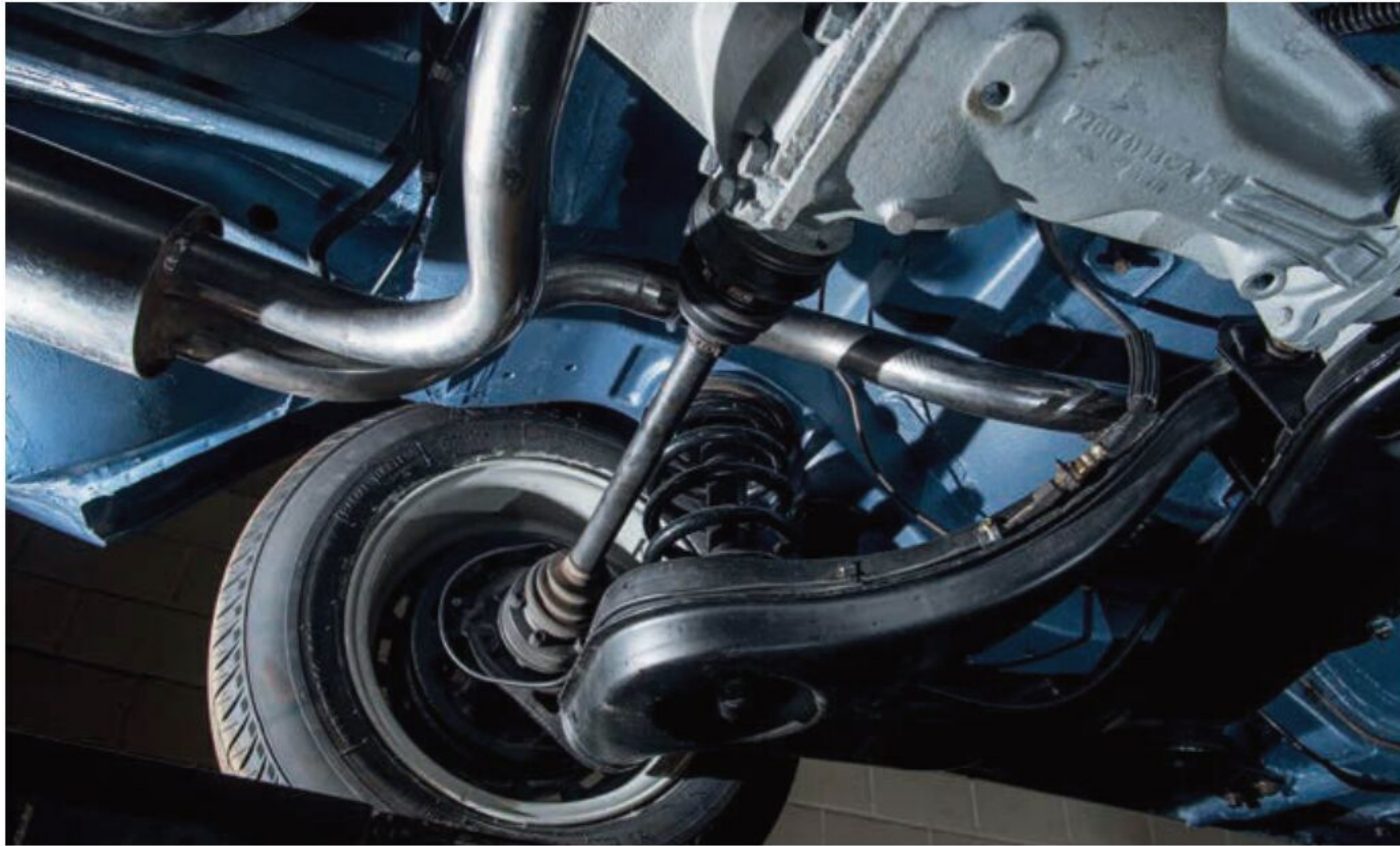
The underside is every bit as good as you'd expect. Stainless steel exhaust carefully follows the pattern of the original.
