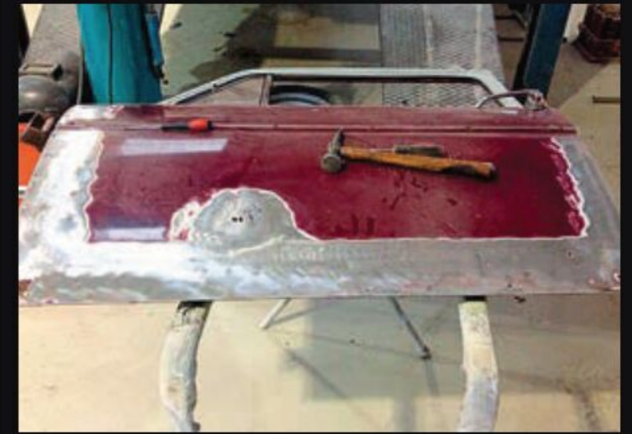
The numerous body repairs included making up and letting in repair sections to the bottoms of both doors.
