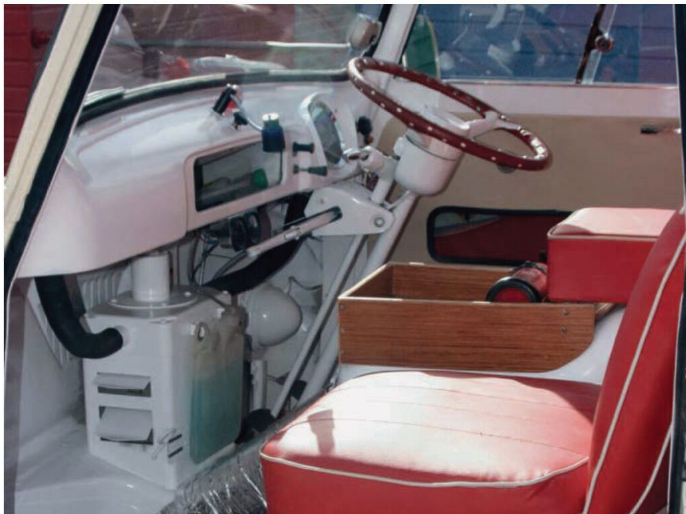
Cab access was good. Heater was optional but is definitely a plus point for year-round use, although in summer the engine alone can make the cab a little too toasty.
