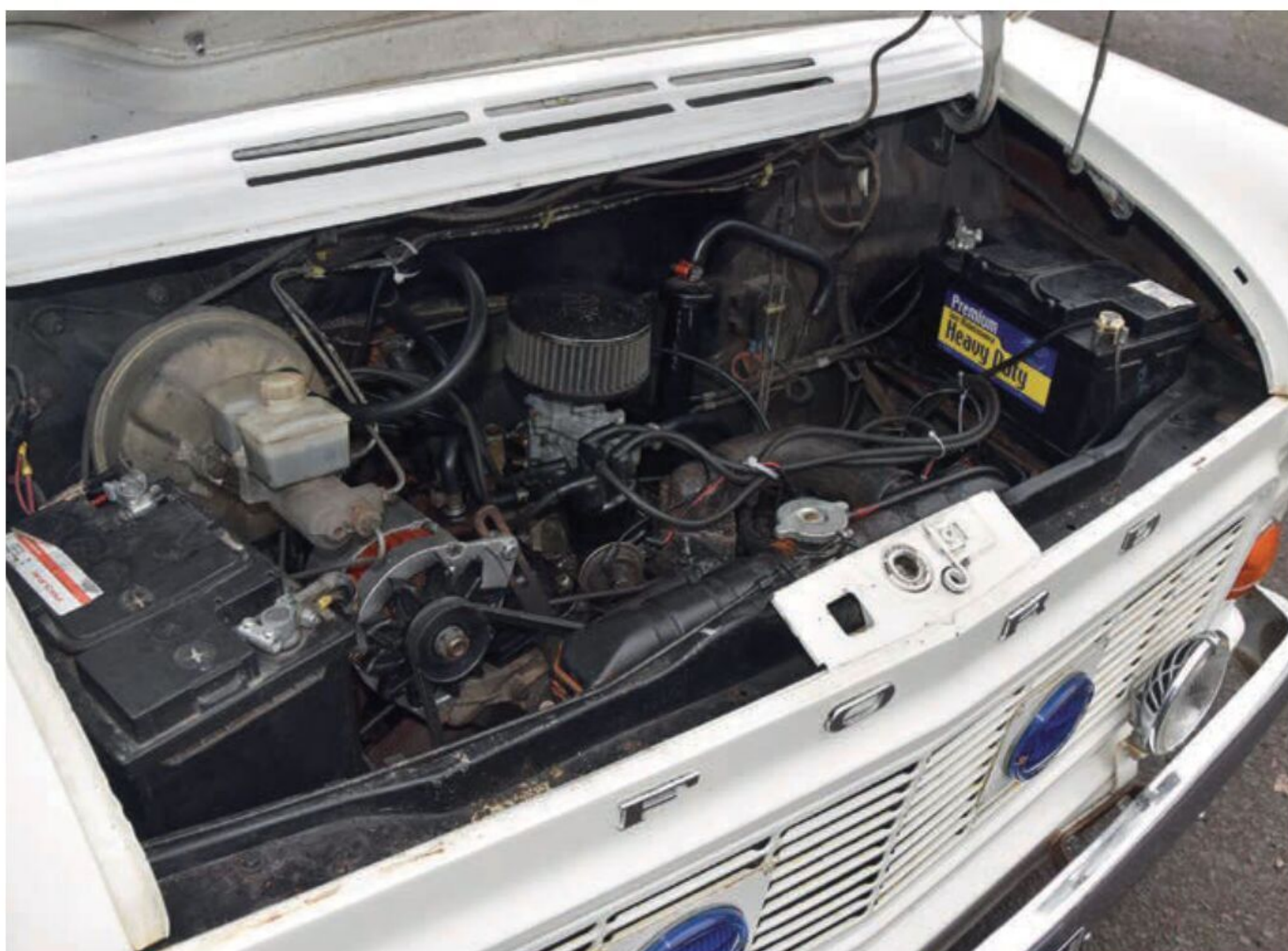
2-litre V4 was the standard petrol offering, though some emergency vehicles actually came with a V6 3-litre unit.
