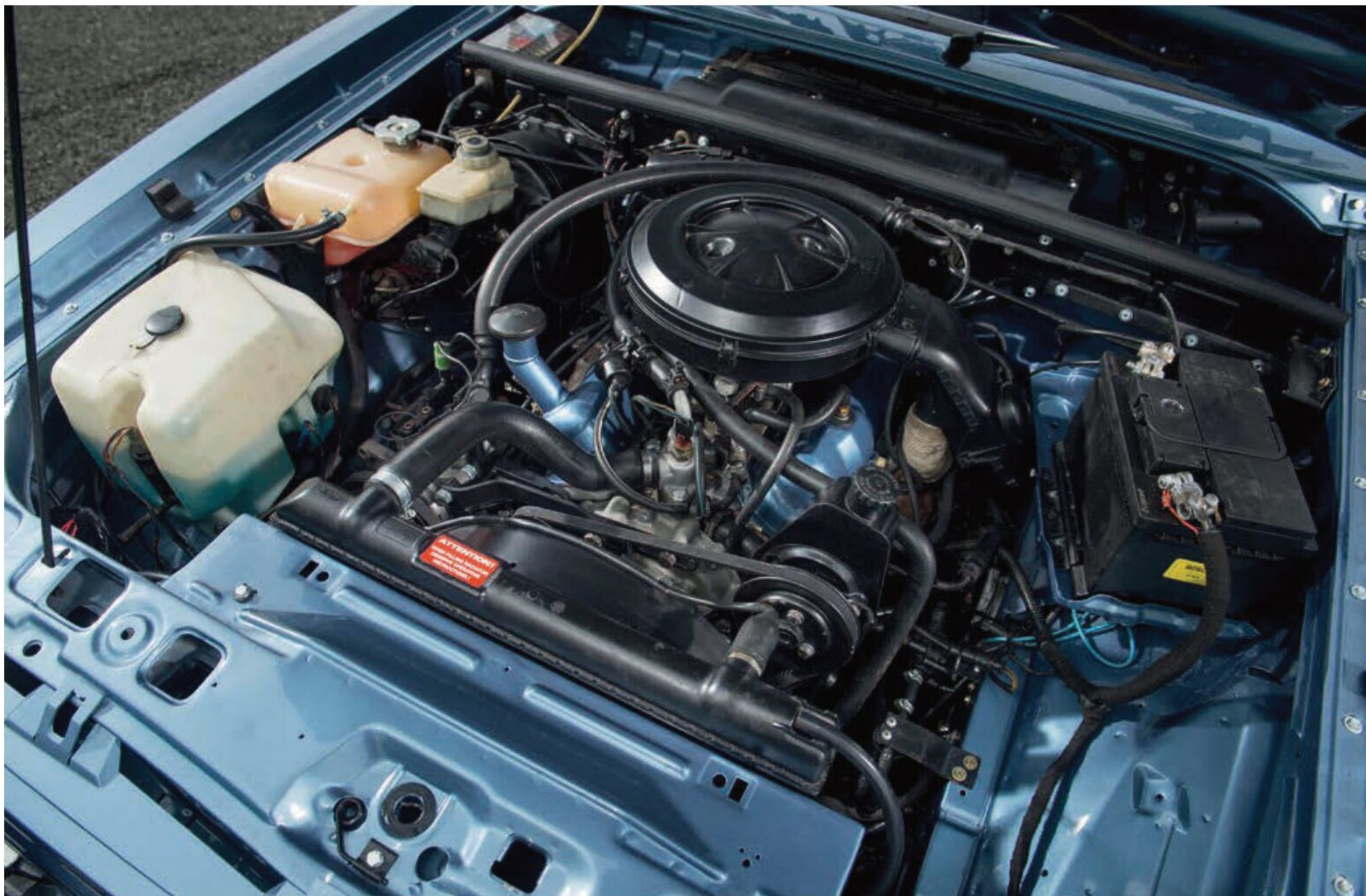
The Cologne V6 had only covered 1500 miles but was still stripped and checked as a precaution — then fully detailed.
