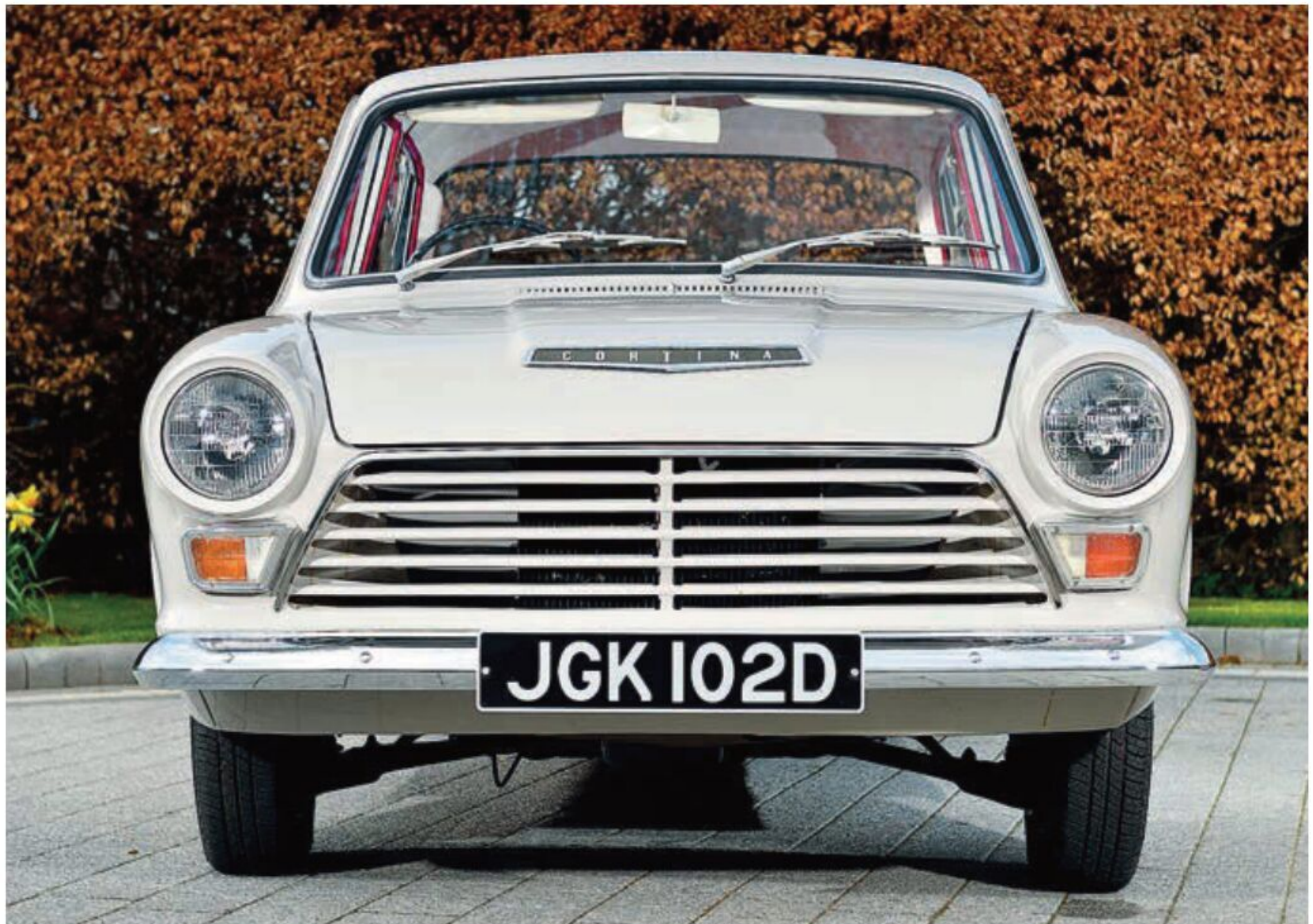
Slatted front panel is unique to the base/fleet models.
