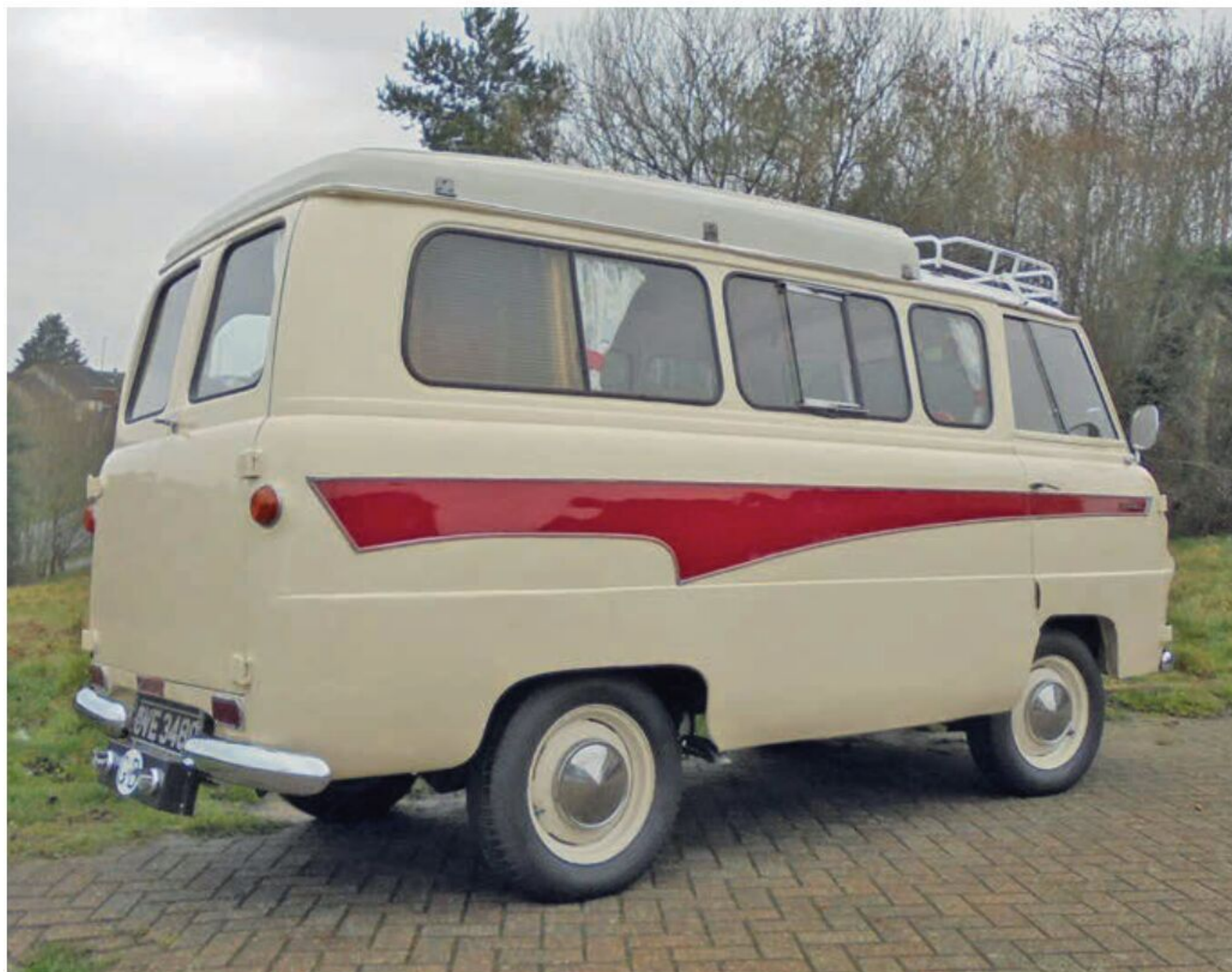
The forward-control layout was designed to maximise payload within the overall length.
