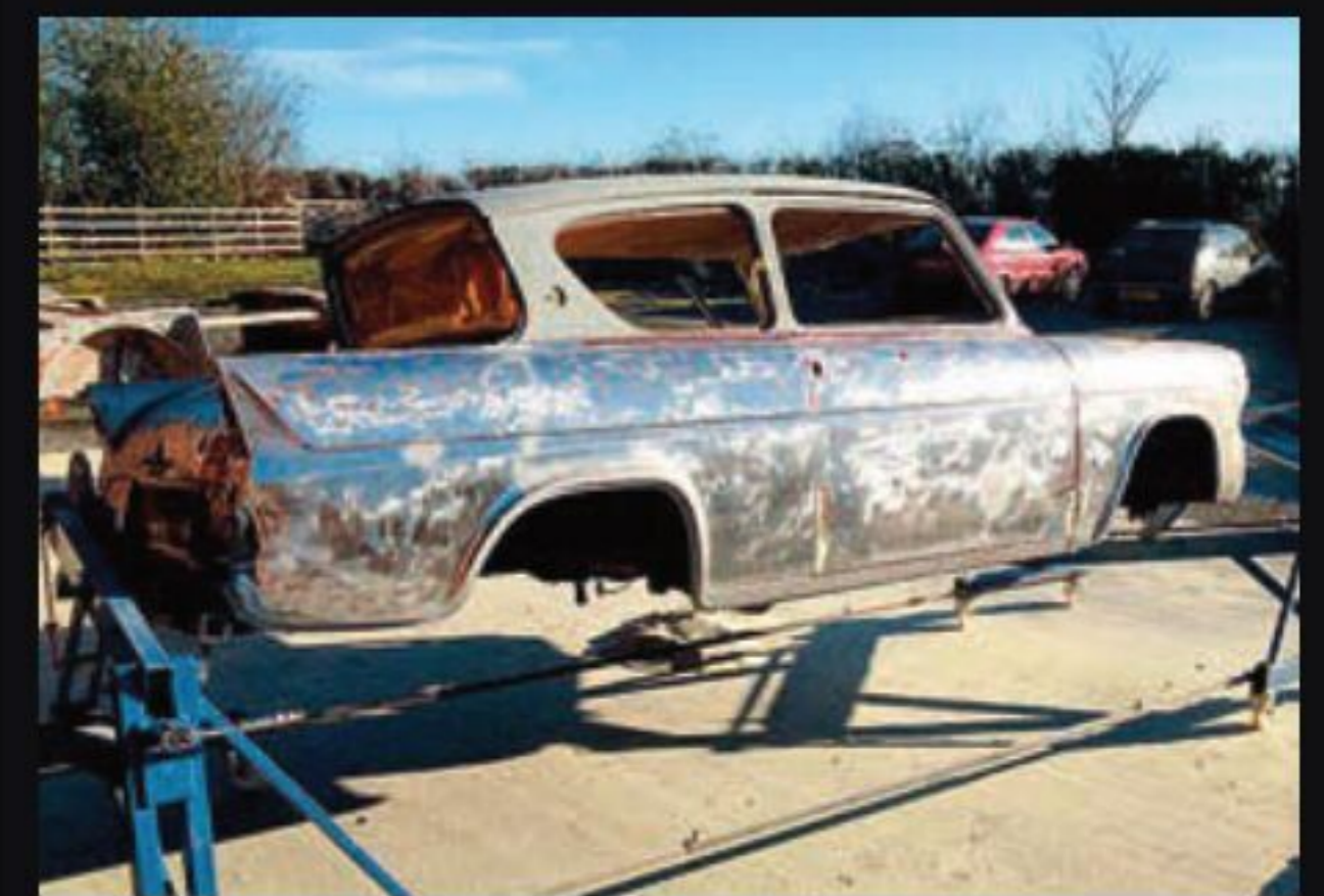
The Anglia shell was stuck on a spit and blasted to a bare shell everywhere except the boot.
