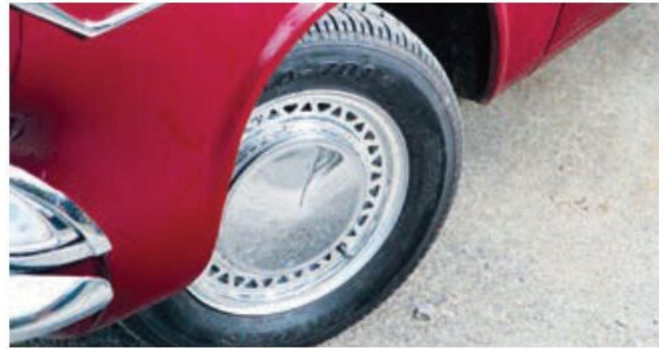
Standard skinny steels hide the original drum brakes.
