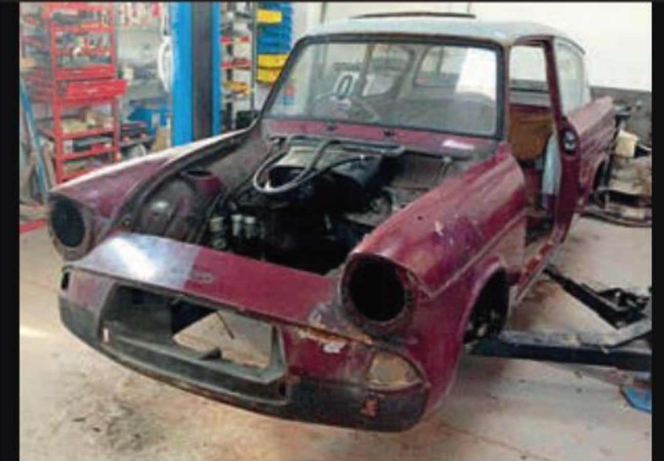
First task was to strip the Anglia right down to a bare shell in Longmynd's dedicated workshop.
